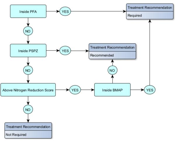
*Figure 4.* Flow chart with queries to identify where OSTDS upgrades to AWTS or connection to central sewer are required.
