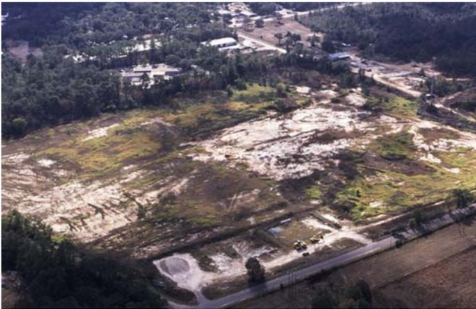
The primary sediment disposal site was designated as the County's Eisenhower Clay Pits, approximately five miles from Lake Munson and four miles from Lake Henrietta. The site is a former clay borrow pit and an active municipal fill pit with 600,000 cubic yards of storage capacity. A site plan was developed to ensure that no stormwater runoff left the site. This assisted in addressing concerns from adjacent residents regarding impacts from the fill activity.
