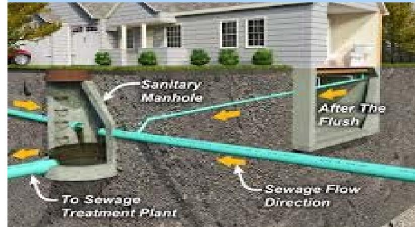
Wastewater flows from house into closed gravity piping system and is pumped to WWTP for treatment.
