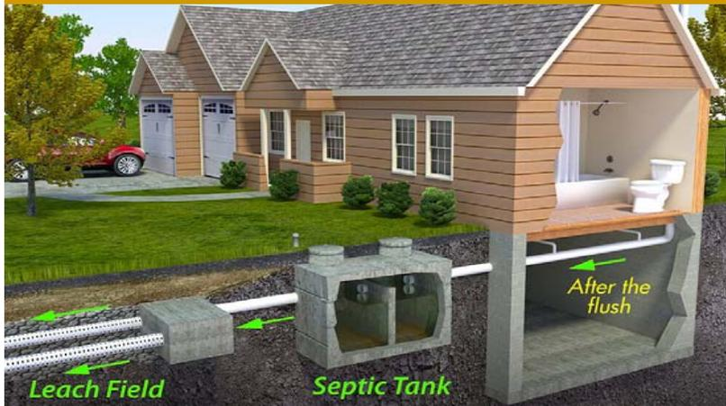
Wastewater flows from house through septic tank and drain field into the soil and groundwater and surface water.
