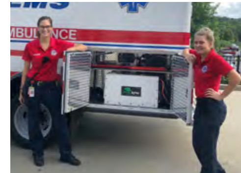
On-board battery systems installed on EMS ambulances
